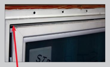
**Window without Corner Drive:**Noticeable separation in top corner of window at DP75
